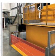
▲ Light Beam Exclusion Zone Stops lift if goods/person enters
