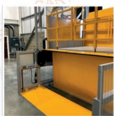
▲ PVC Blinds Extra safety under lift platform
