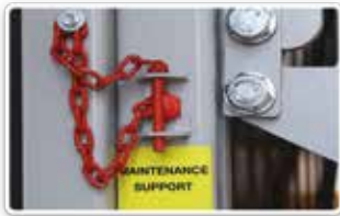
MAINTENANCE SAFETY PEGS: EASILY ACTIVATED FOR SAFE SERVICING
