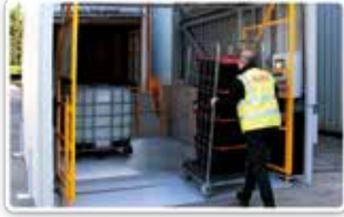
FIXED, SHALLOW LEAD-ON RAMP – SPEEDS UP LOADING AND MINIMISES MANUAL HANDLING
