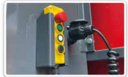
▲ Controls Lift can be operated from platform or ground level
